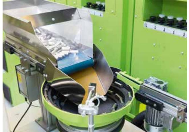
**Fig. 2.** "Green" Liquidmetal parts are singulated automatically, and then fed to the melting chamber (figure: Engel)
