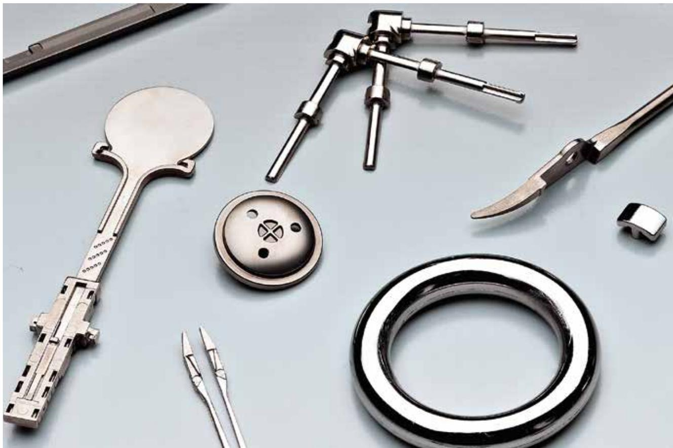
The Liquidmetal process permits extremely fine structures to be produced efficiently by means of injection molding (figure: Liquidmetal Technologies)
