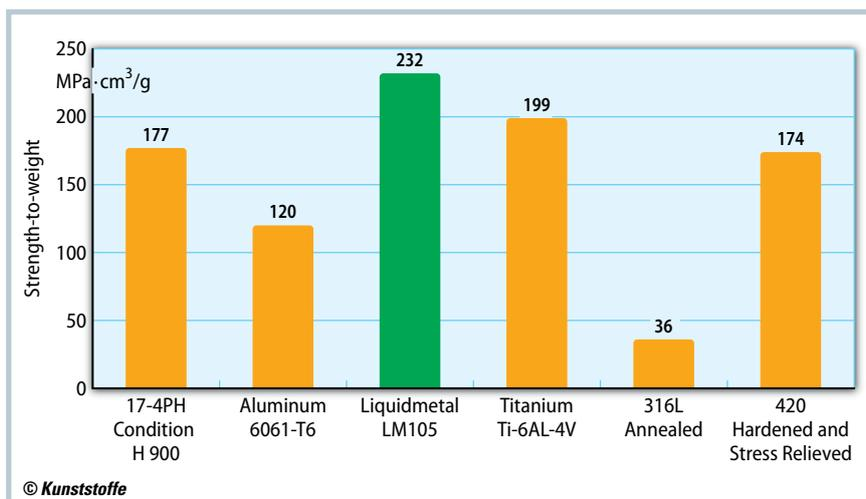
Fig. 4. Strength/weight ratio: The metal alloys permit the production of extremely robust components with a comparatively low weight (steel type descriptions acc. to US standards)
