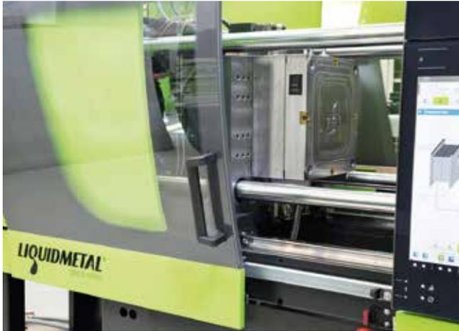
**Fig. 1.** The new injection molding machine is based on a fully electric Engel "e-motion" (figure: Engel)
