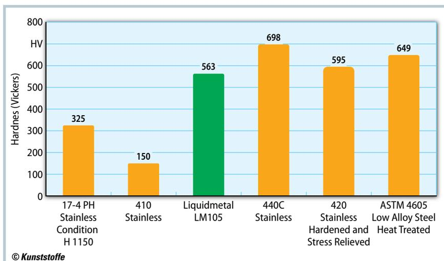
Fig. 5. Contrary to Liquidmetal, steels require extensive post-production thermal treatment to obtain a high Vickers hardness (steel type descriptions acc. to US standards)
