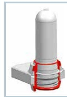
New self-cleaning technology makes it possible to clean molds (affected zones shown in color) in seconds instead of hours at the touch of a button (figure: Husky)
