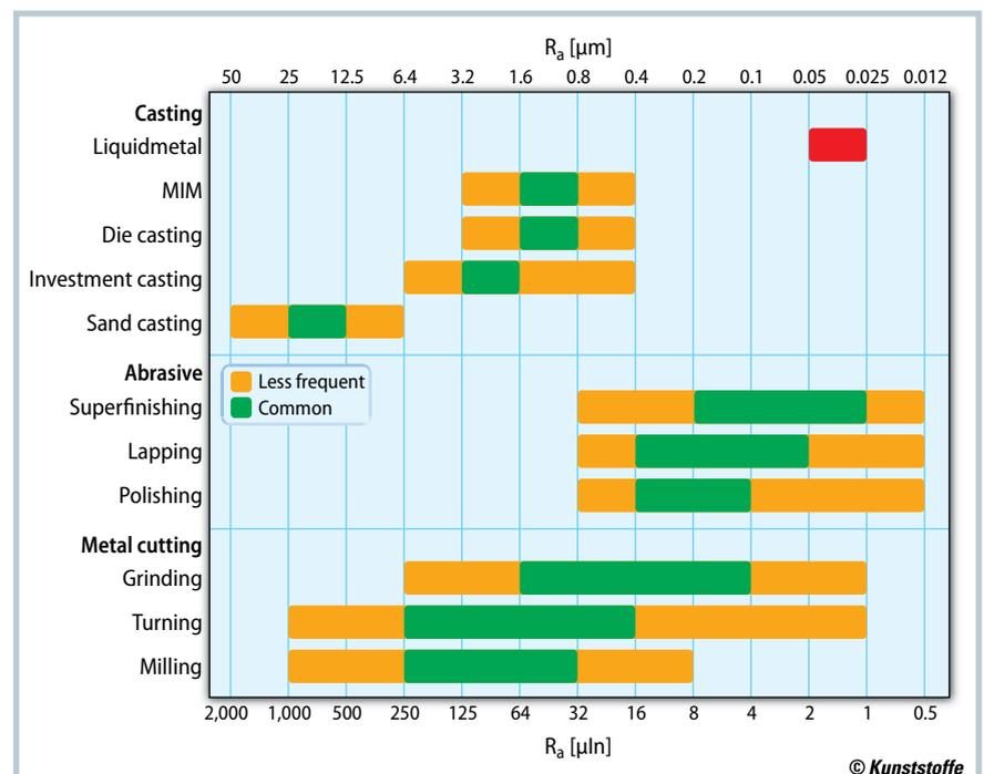
**Fig. 3.** The Liquidmetal process creates components with high surface quality that require no rework, and its high efficiency sets it apart from alternative methods (source: Liquidmetal Technologies)
