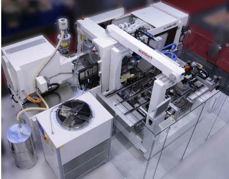
Fig. 1: Production cell with ENGEL e-motion T for manufacturing pipette tips (r.).
