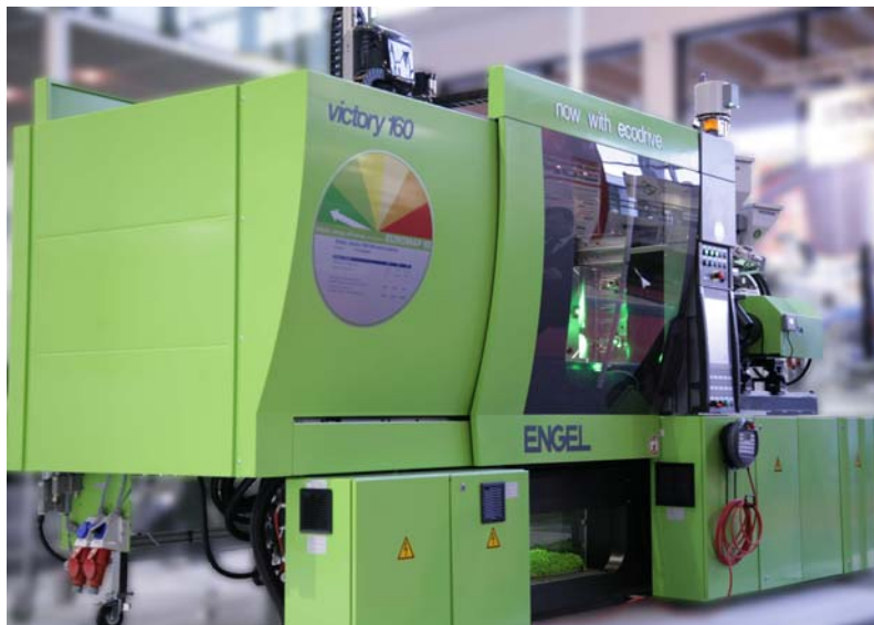
Fig. 2: ENGEL victory 160 with ecodrive for manufacturing a bearing block for sanitary applications (r.)
