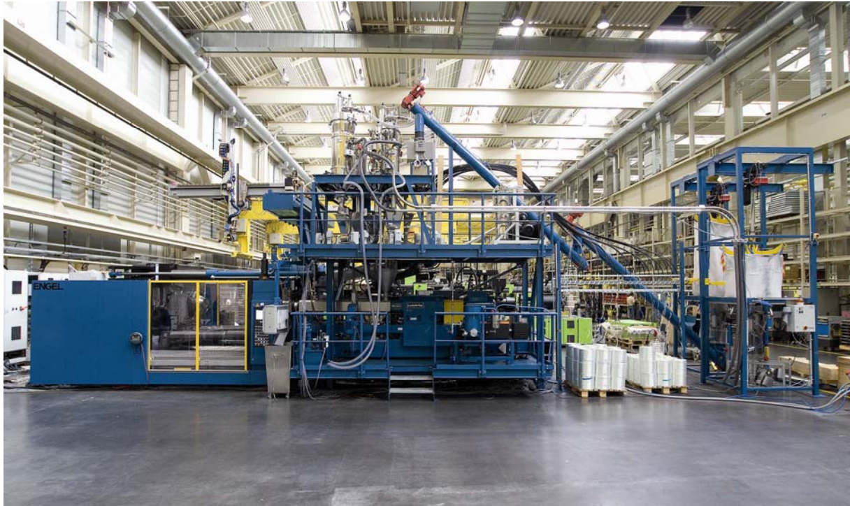
Fig. 1: ENGEL injection-moulding compounder with an integrated ZSE MAXX extruder of Leistritz.
