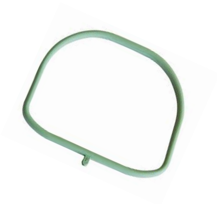
Seals, manufactured on an ENGEL elast 280/150 VC rubber injection moulding machine with tiebar-less clamping unit and a 16-cavity mould by Ro-Ra Produktions GmbH
