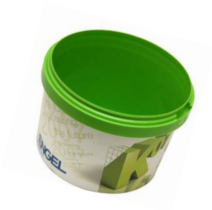
Round polypropylene cups with original product seal, produced and decorated with a cycle time of 3.7 seconds in a 2-cavity mould at K 2007 by means of in-mould labelling on an ENGEL speed 180/55
