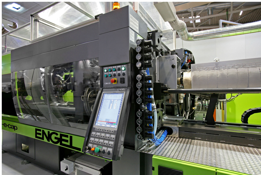
Picture 2: The new ENGEL e-cap machine – the first fully electric cap-production solution
