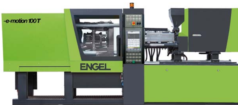
Picture 2: ENGEL e-motion 100T for the manufacturing of PP pipette tips
