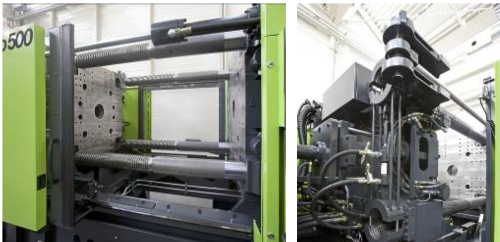
Fig. 3: Easy access to the mould area from the operator and non-operator sides
