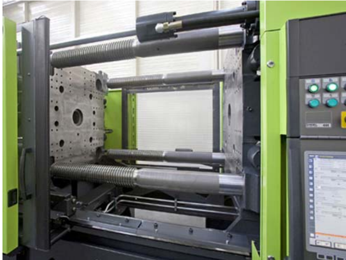
Photo 1. ENGEL offers the only two-platen injection molding machine that has no contact with the tie bars, allowing frictionless movement to better control speed and precision.
