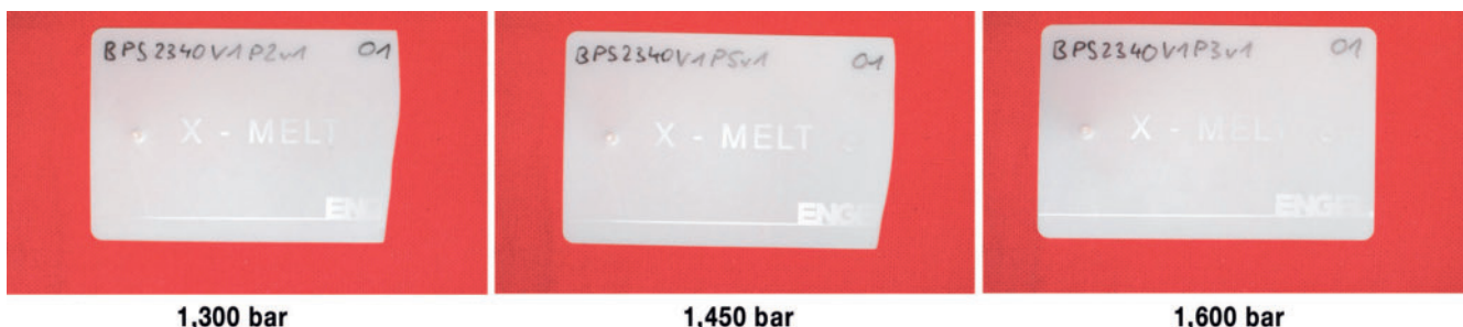
Fig. 5. The photos of check card parts photographed at different compression pressures show that the cavity was completely filled at 1,600 bar
